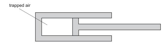
The piston is moved so that the pressure of the trapped air increases by 20%. The temperature of the trapped air does not change.
